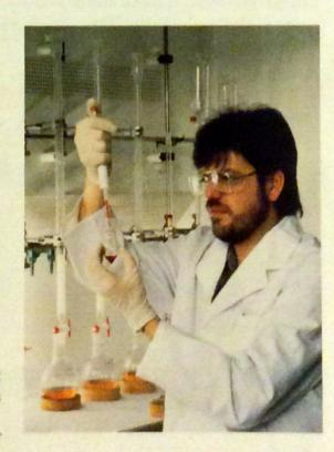
A pipette is used to measure a known volume of liquid accurately. Burettes and conical flasks, which are also used in the titrations, are in the background.
