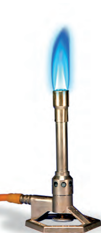
The Bunsen burner controls the combustion of methane, \text{CH}_4 , and is often used as a source of heat in the laboratory.
